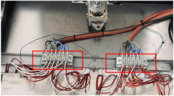
10) Finally, remove the cover plates, insulation and you can replace the heating elements
