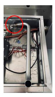
8) Disconnect the waste engine from the pins and unscrew the motor bracket
