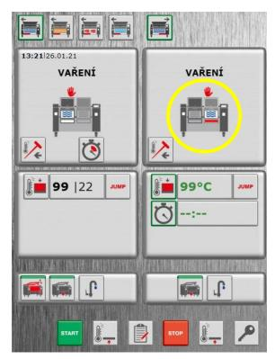
5) If one half of the pan drowning differently than the other half of the pan, you can adjust it with the values in **L plate** and **P plate**
